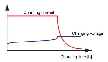
First, the grid|power FNC® cells are charged with a constant charging current. The maximum current has to be limited to  $\leq I_5$  (e.g. for a 100 Ah battery the current  $I_5 = 20$  A).
