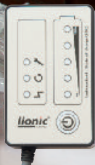
Fig. 13: External charge state and status indicator
