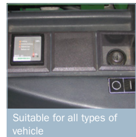
Battery Control Unit (BKE)
