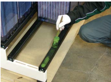
Fig. 5-12: Lubricated support profiles
