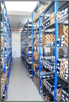
520 mm D x 1000 mm W x 2997 mm H with each bay comprising 7 levels + 11 bays of 420 mm D x 1000 mm W x 2997 mm H with each bay containing 7 levels + 2 bays of 420 mm D x 1000 mm W x 2997 mm H with each bay containing 6 levels + 1 bay of 420 mm D x 1000 mm W x 2997 mm H with each bay containing 4 levels. The total number of shelving locations adds up to 431.
