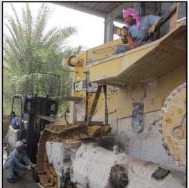
seals were found collapsed and damaged. The assembly and installation was carried out as per **Caterpillar** specifications and torque values. Each step was doubly checked and verified to ensure that there was no room for any error.
