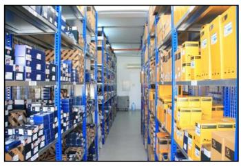
bays of 900 mm D x 2700 mm W x 2400 mm H + 1 bay of 900 mm D x 1350 mm W x 2400 mm H with each bay of 4 Levels have been installed to carry the heavier and / or bulky parts. Each bay has a pair of beams, providing a total racking of 20 locations.
