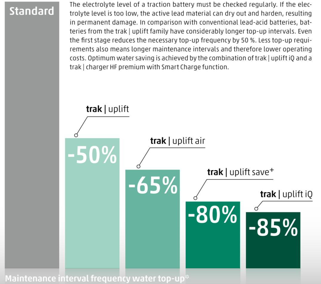
\* Max. servicing intervals can only be achieved in combination with a trak | charger HF premium and an appropriately adjusted charging curve. The standard corresponds to charging with CF 1.2.
